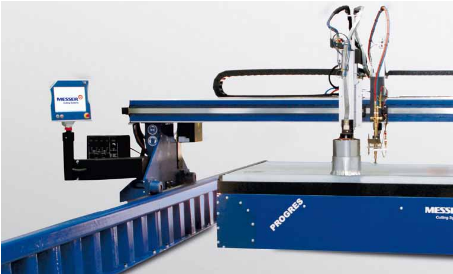
The modern cnc control Global Control and the plasma interface are mounted where the operator can easily see and adjust them.
