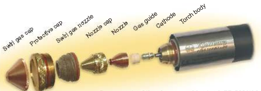
Components of the plasma machine torch PB-S80 W-2
